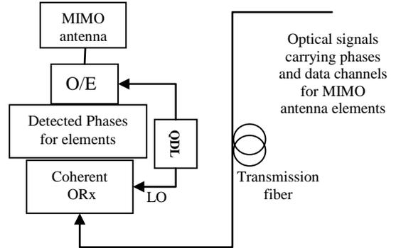
Figure 3: Delivering phase and data info to MIMO antennae for 5G wireless networks.
