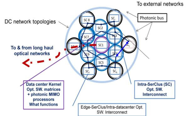
Figure 8: DC structure with a photonic kernel at the center and satellites of clusters of servers.
