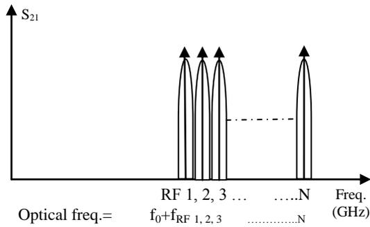
Figure 5: RF frequency spectra and equivalent resonant optical frequency responses for optical modulators for several MIMO antennae systems.  $f_0 = 193.51$  THz (1550nm or equivalent for 1310nm).
