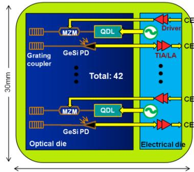
Figure 2 Integration of QDL on Si-IP optical transponder.
