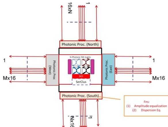
Figure 6: Structure of a photonic kernel of DC in 5G networks.
