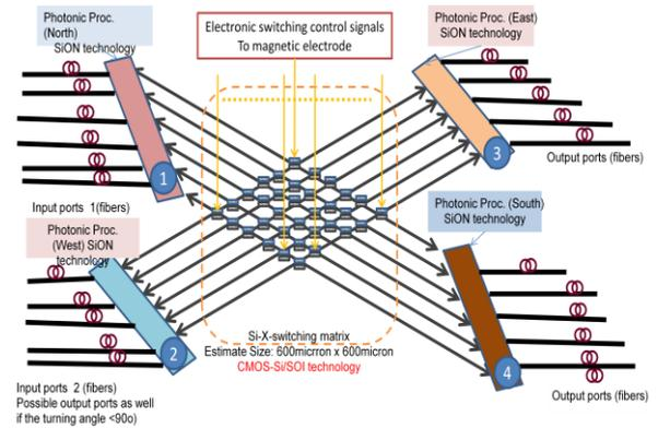
Figure 7: Photonic switching matrix
